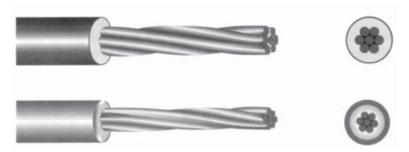
The above wiring cables conform to BS 6004 specification for "PVC insulated cables (non-armoured) for electric power and lighting". The cables also generally satisfy the International Specification IEC 60227 (6491 X only) and German standard VDE 0281 for "PVC insulated cables and cords with rated voltage not exceeding 750V"
